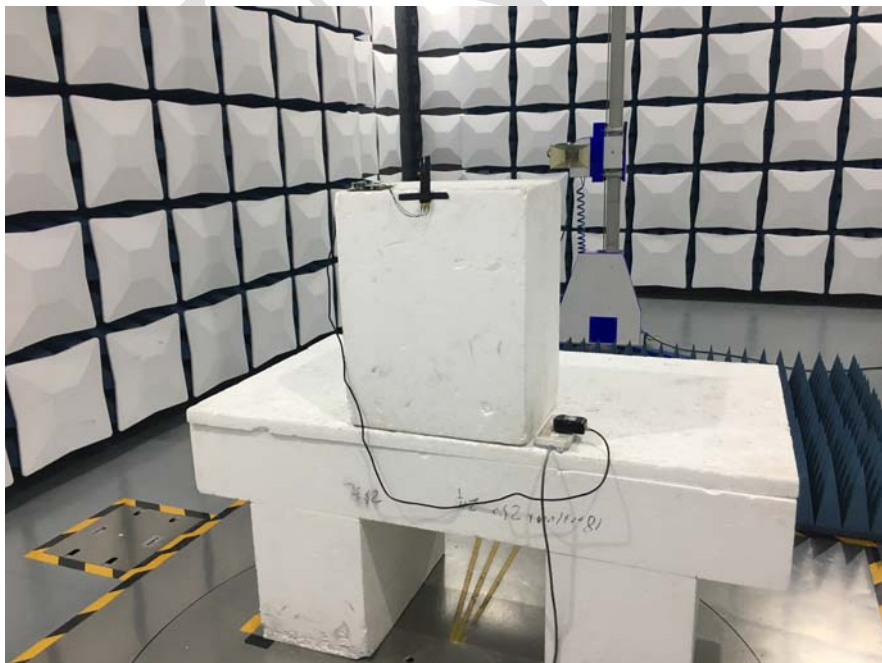
Radiated Spurious Emissions Test View (Above 1GHz)
